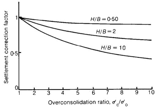
**Fig. 10. Settlement correction for three-dimensional effects on initial excess pore pressure distribution (adapted from Highway Research Board, 1973)**
