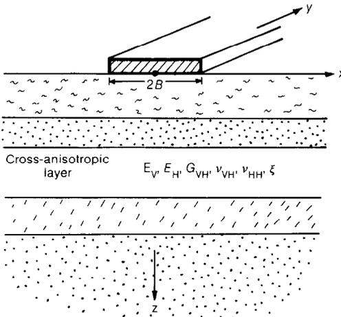
Fig. 1. Soil profile and footing diagram
